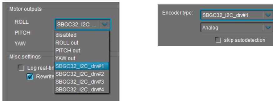
3. It's better to increase the I2C speed by selecting the “I2C high speed” option in the “Hardware” tab, to minimize delays caused by the I2C data transfer. But it may be required to decrease overall resistance of pullups on SDA, SCL lines to 1..2k, otherwise I2C errors may come. Please pay attention to this fact when designing your own system.
